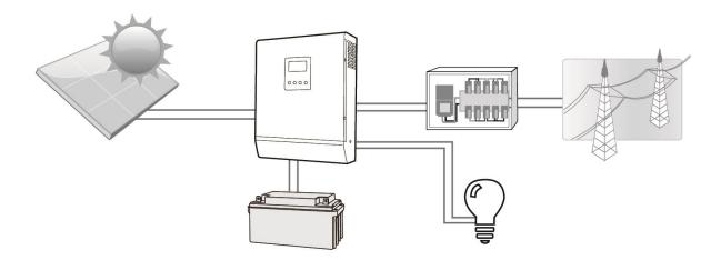
Figure 1 Basic hybrid PV System Overview
